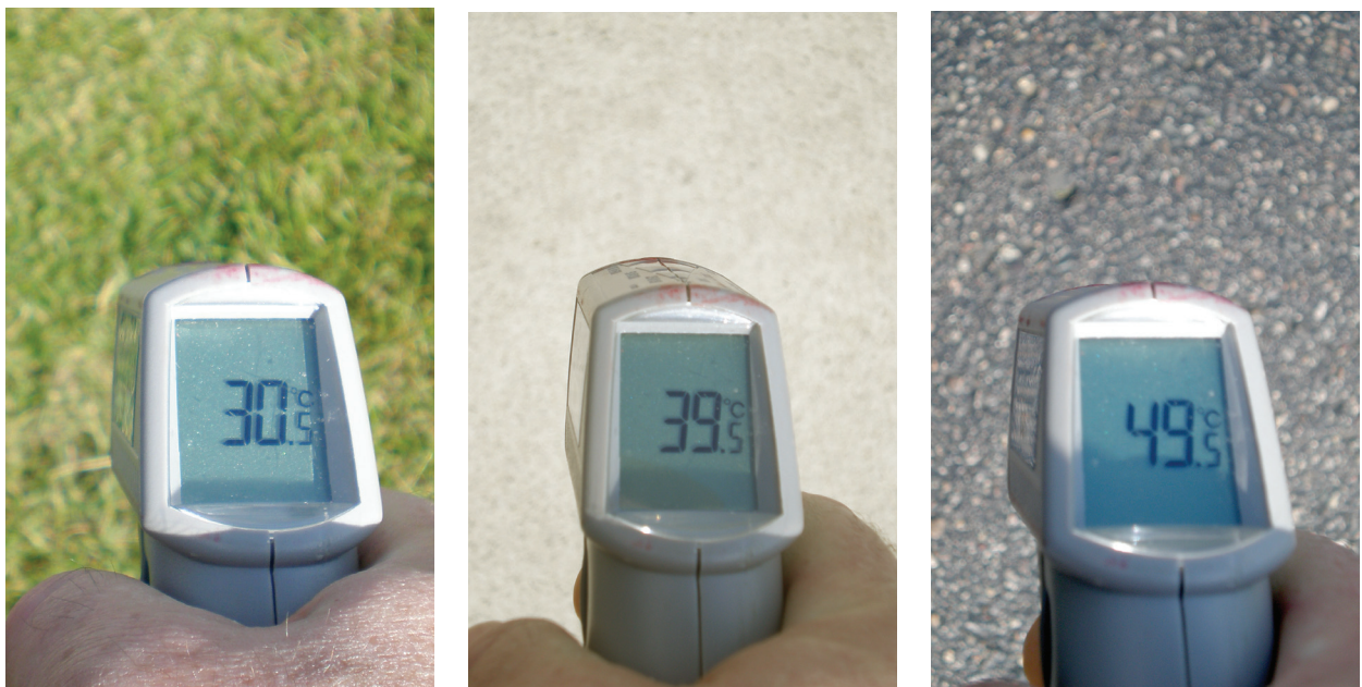
Fig. 2.38—Grass, concrete pavement, and asphalt pavement surface temperatures measured using an infrared thermometer. These readings, taken within meters of each other on same spring afternoon, demonstrate effects of transpiration and solar reflectance on surface temperatures. Grass remains cool because it reflects some solar energy and sheds heat by evaporative cooling. Concrete pavement remains cool because it reflects solar energy very well, but asphalt pavement reaches high temperatures because it absorbs almost all incident solar energy.
