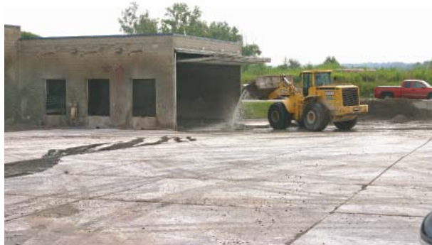
Fig. 1.3—On-site water treatment at a ready mix facility in Burnsville, MN: (a) the first three stilling basins are shown herein. The fourth runs along the rear of the structure transverse to the others. Note the berm used to direct site runoff into the first basin; (b) view into the facility showing the froth on the water in the first basin. This material will break up overnight. Solids need to be removed frequently; (c) cleaning is readily done with a front-end loader. Solids are reclaimed as fill; (d) water passing the weir from Basin 1 to Basin 2. The weir is baffled to hold back the froth. Note the lack of froth in Basin 2; and (e) the finished water in Basin 4. The material on the surface is calcium carbonate, resulting from CO_2 sequestration from the air. The water at this stage has a pH of 12.5 but very low suspended solids. Photos courtesy of Cemstone
