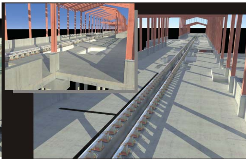
Fig. 2.8—Concrete and steel tolerance model. Rendering courtesy of Virtual Design & Construction Dept., KLORMAN Construction
