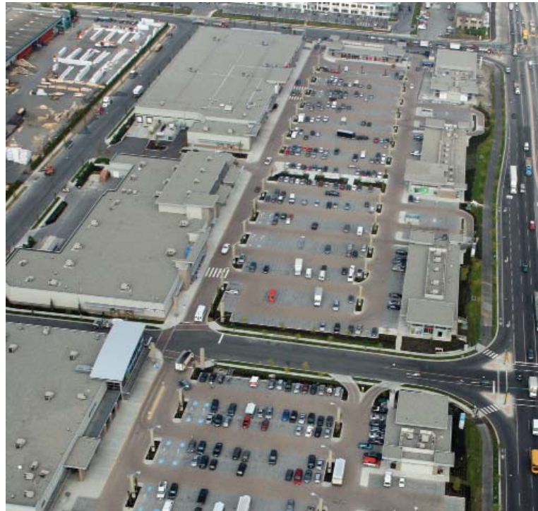
Fig. 3.38—With no space for a separate detention pond, the permeable interlocking concrete pavement parking lot becomes the detention facility for roof and parking lot runoff. Photo courtesy of Interlocking Concrete Pavement Institute
