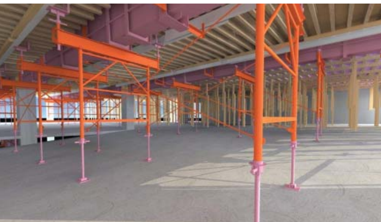
Fig. 2.4—Rendering of suspended slab formwork systems used during construction. Rendering courtesy of Virtual Design & Construction Dept., KLORMAN Construction
